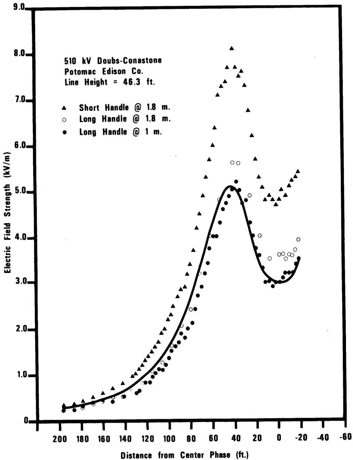
FIGURE 1. ELECTRIC FIELD STRENGTH PROFILES USING A POLYTECH FBM-100
