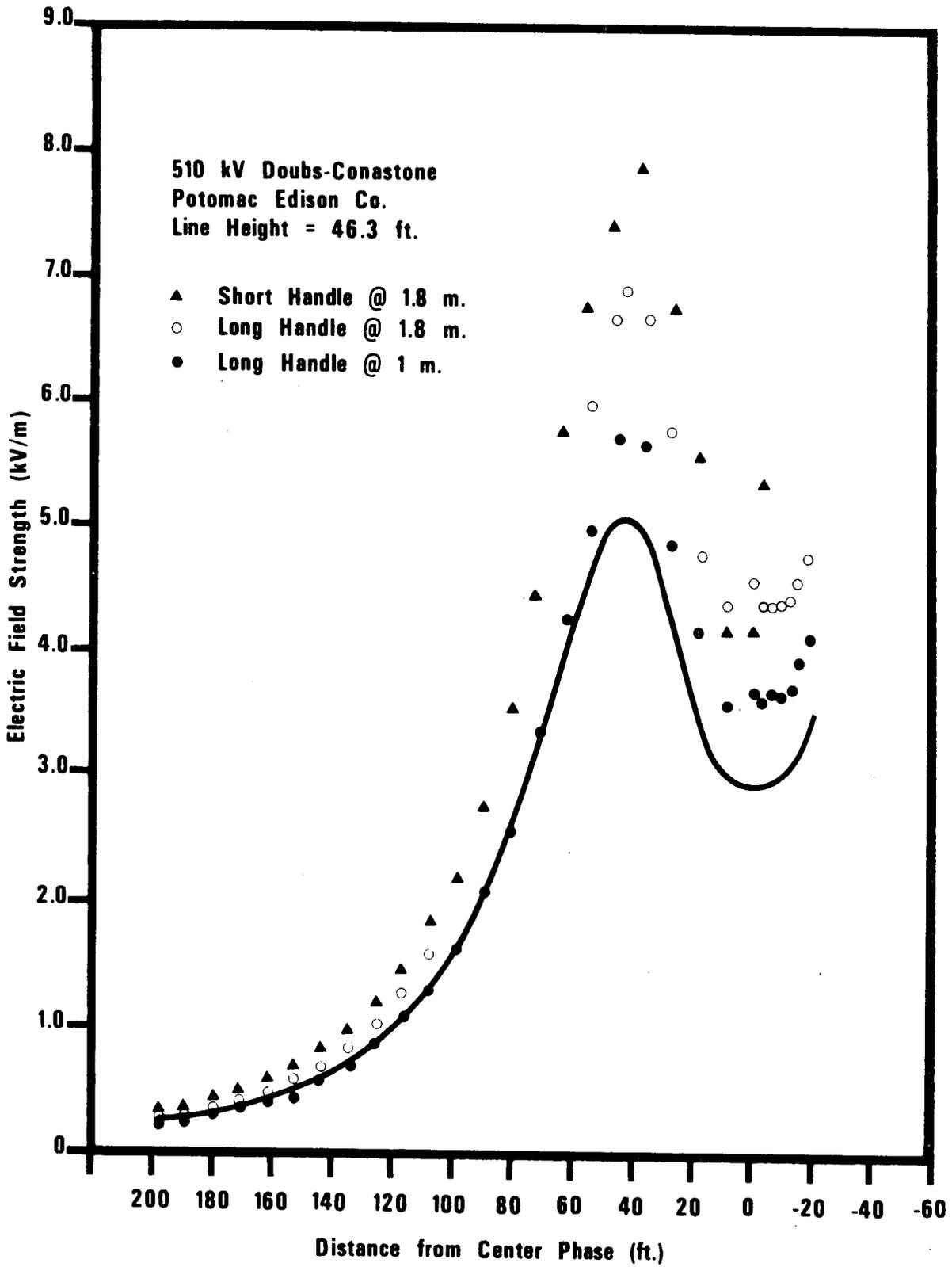
**FIGURE 2. ELECTRIC FIELD STRENGTH PROFILES
