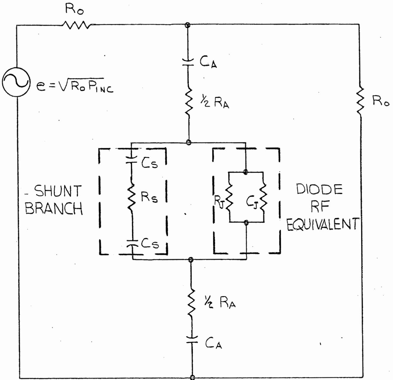
Fig. 1. Resistive Probe RF Schematic
