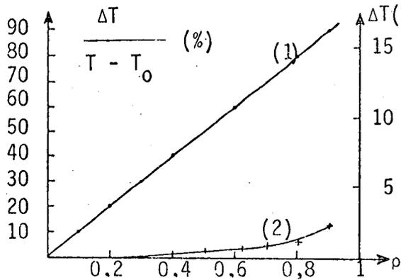
Figure 4 - Relative error on measured temperature versus  $\rho$  and absolute error  $\Delta T$  for T = 38°C
