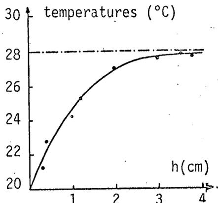
Figure 1 - Radiometer signal in the case of short circuited waveguide cell (thickness h) with chloroform at 30°C (f = 9 GHz)
