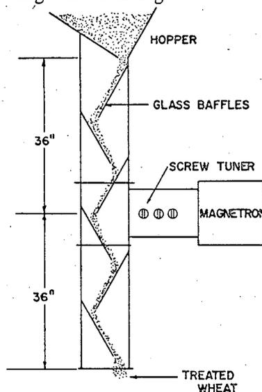
FIG. 1. First design for the control of insects in wheat circulating through a waveguide.
