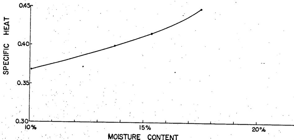
FIG. 3. Specific heat vs. moisture content of wheat.
