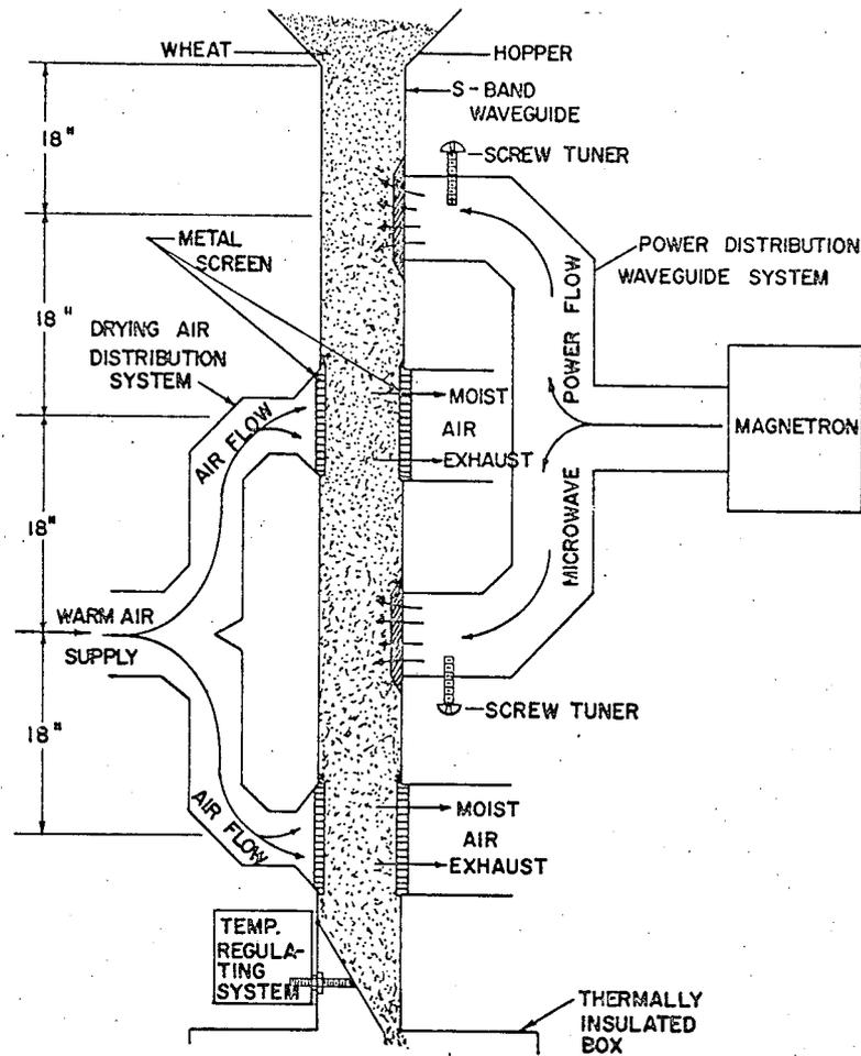
FIG. 7. Practical system for control of insects in wheat and flour and drying of grain.
