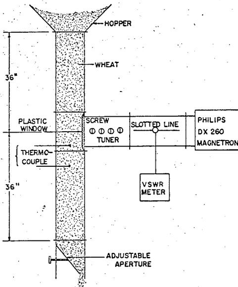
FIG. 2. Final design of the microwave system used for the control of wheat insects.
