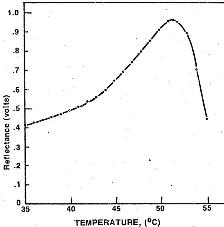
Figure 9 Reflectance as a function of temperature illustrating the drop in reflectance as the liquid crystals begin to clear at approximately 52°C.
