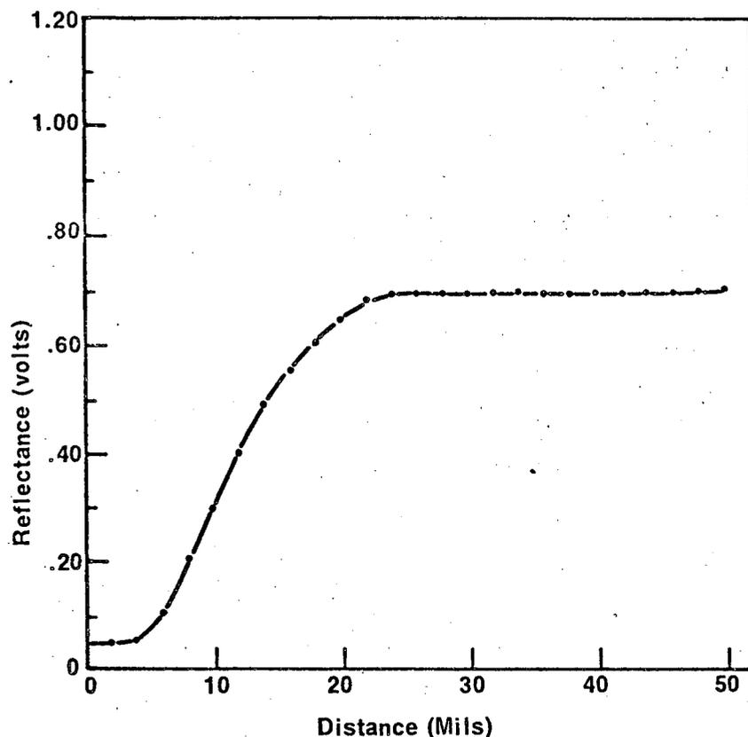
Figure 7 The relationship between the liquid crystal-optic fiber separation and reflectance (R).
