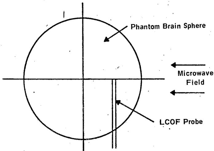
Figure 2 The LCOF probe mock-up is placed in a phantom brain sphere as shown to test for temperature perturbation effects as sensed by the thermographic camera.
