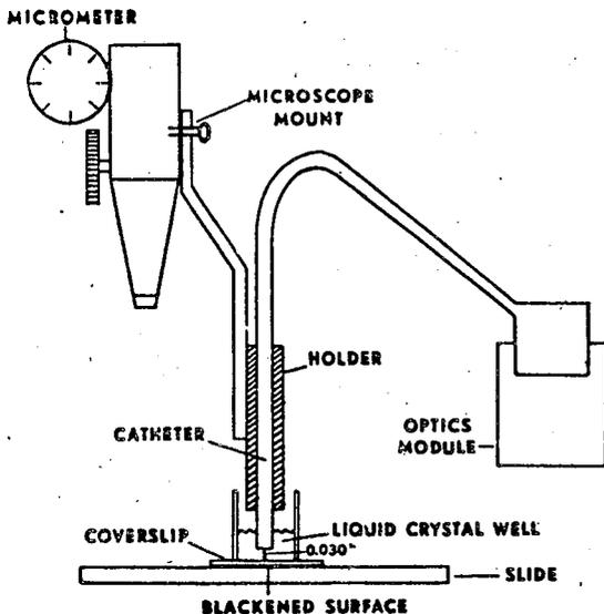
Figure 6 Apparatus used to determine the relationship between liquid crystal thickness and reflectance (R).
