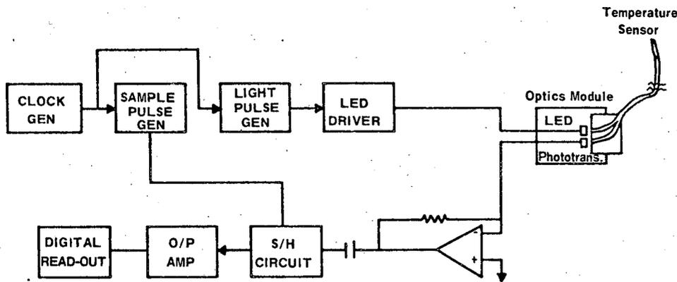
Figure 1 Block diagram of the electro-optical illumination and read-out electronics unit. The temperature probe is connected to the optics module via a snap-in/snap-out connector with position set screw.
