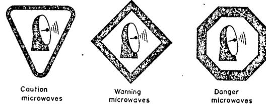
FIG. 3. Three signs to indicate microwave hazards.
