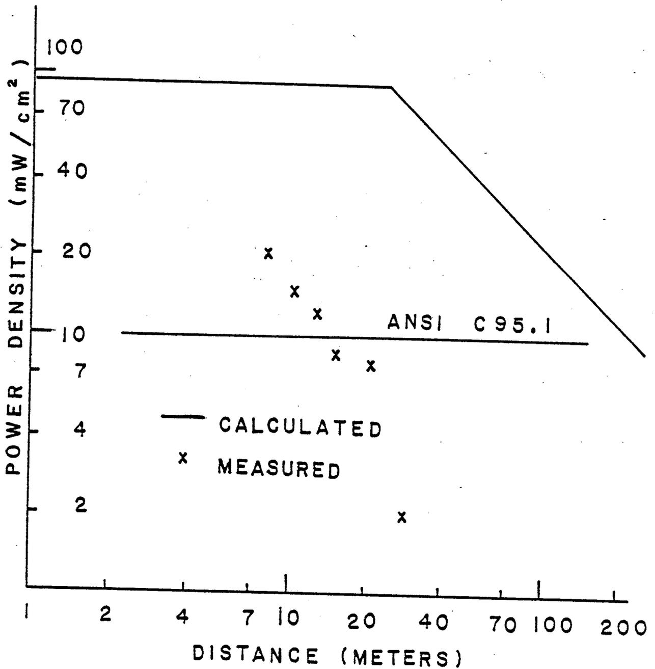
Figure 7 A Comparison of Calculated and Measured Power Densities vs. Distance of a Weather Radar (Enterprise Model WR-100, 5.625 GHz, 157 watts, 6 ft. Dish)
