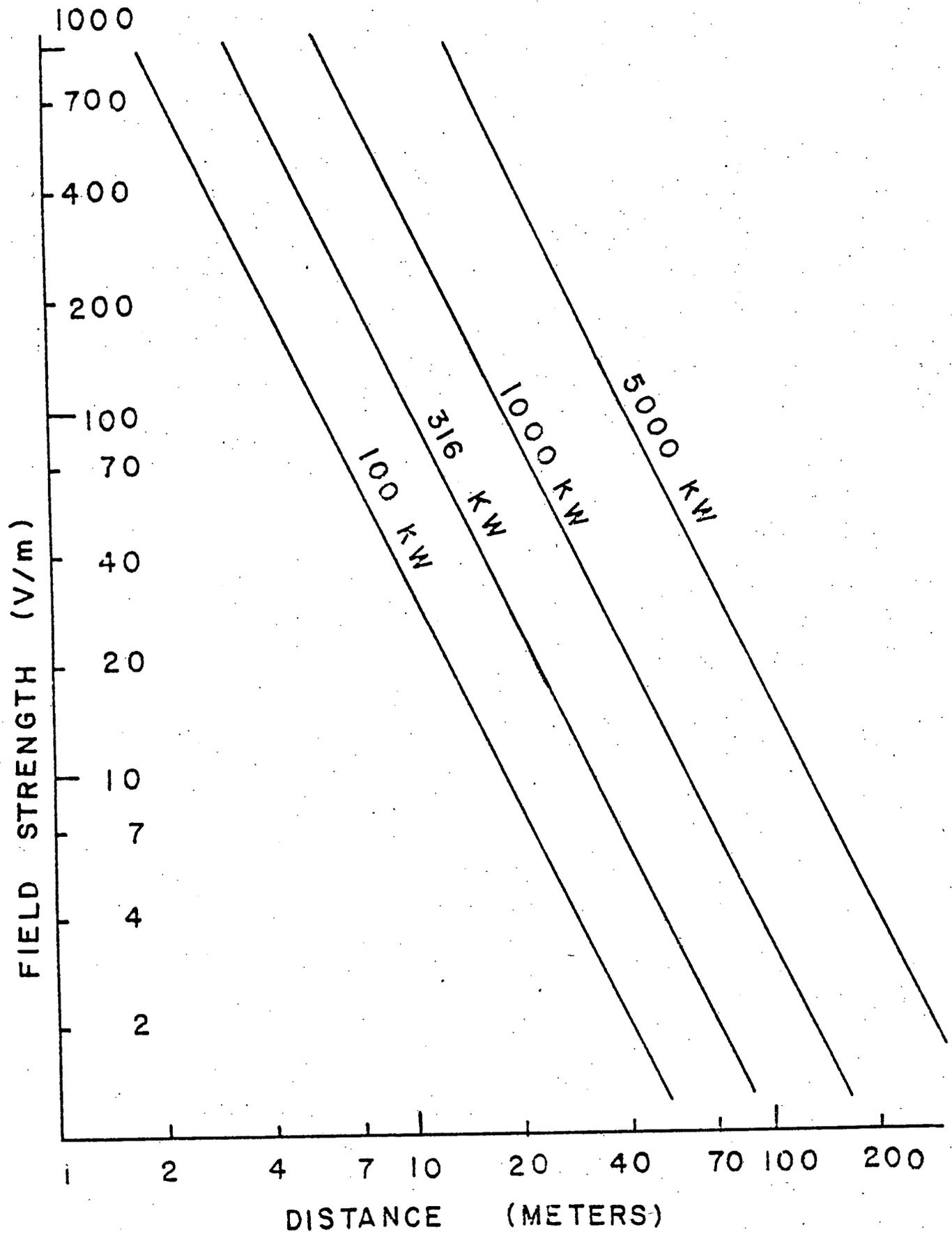
Figure 4 Calculated Power Density vs. Distance for 4 Different Power Levels Used in TV Broadcasting
