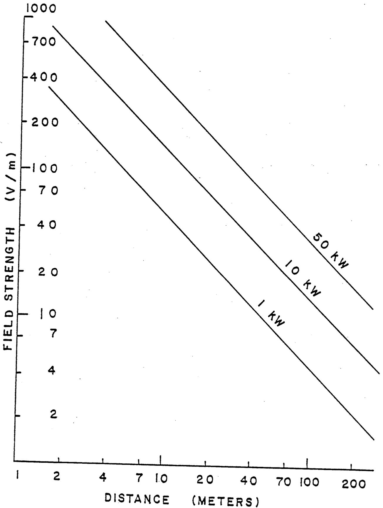
Figure 1 Calculated Field Strength vs. Distance in the Vicinity of a Standard AM Broadcasting Antenna
