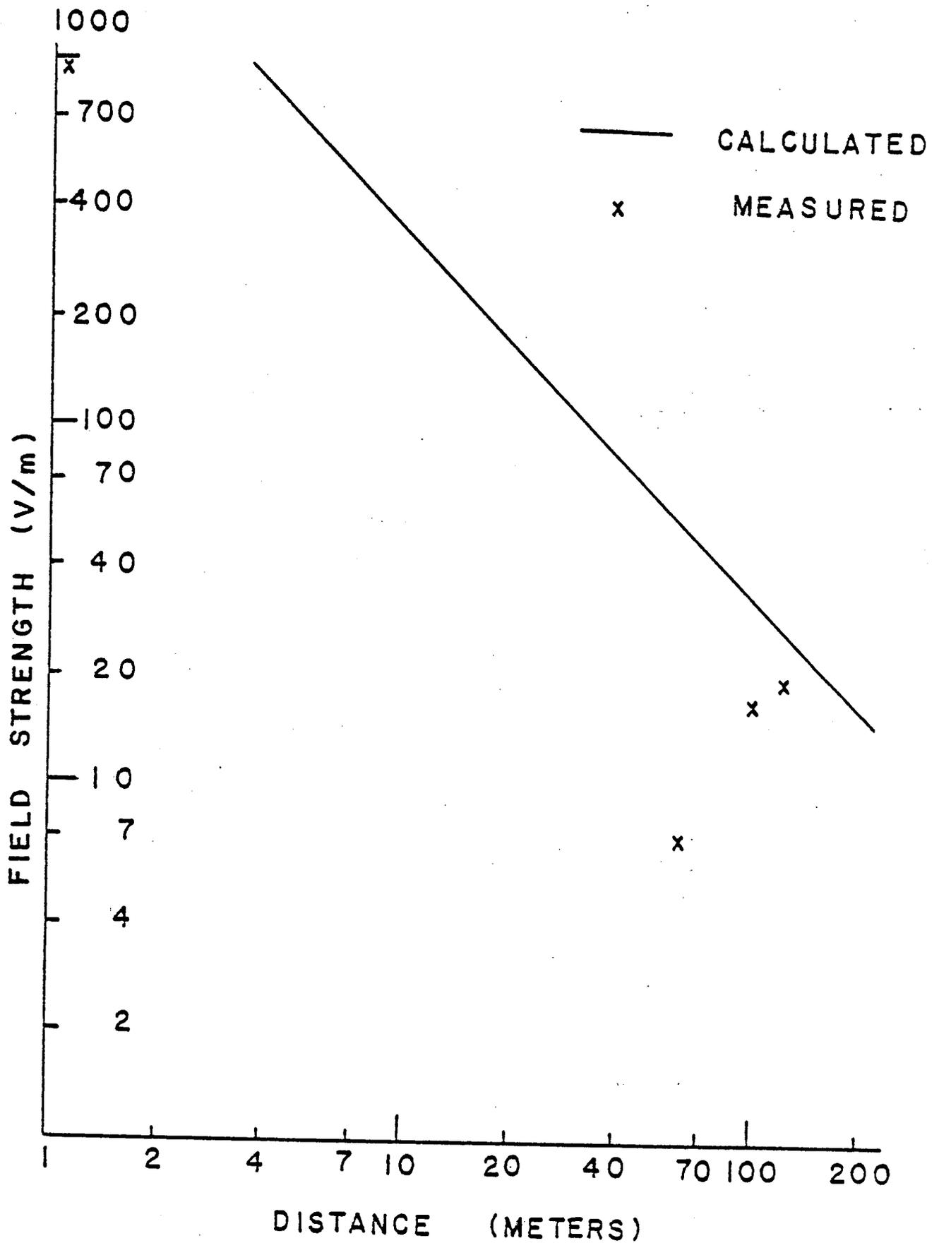
Figure 2 A Comparison of Calculated and Measured Field Strengths in the Vicinity of a Standard AM Broadcasting Antenna (WTOP, Wheaton, MD, 1500 kHz, 50 kW)
