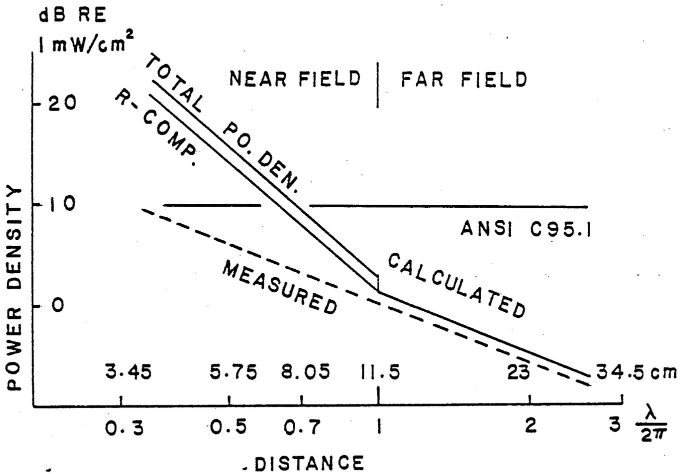
Figure 5 Power Density vs. Distance of a Walkie Talkie (Motorola Model HT-220, 1.8 watts, 415 MHz, see Reference 3)
