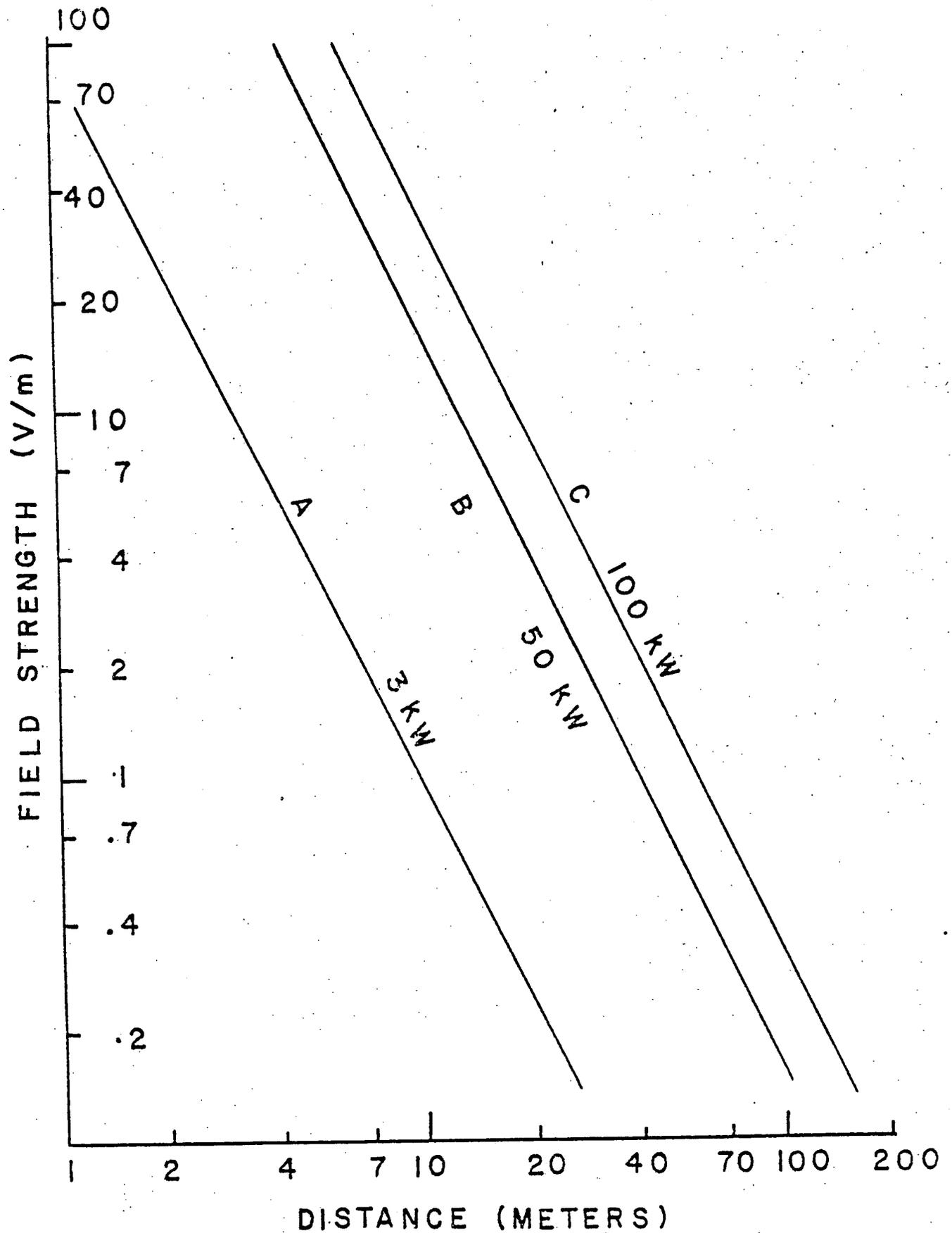
Figure 3 Calculated Power Density vs. Distance for 3 Different Power Levels Used in FM Broadcasting
