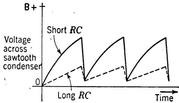
Figure 3—Typical curves showing voltage as a function of time across the capacitor of a series  $RC$  network. Shorter time constant gives higher amplitude, but poor linearity. Longer time constant allows better linearity, but lower amplitude.
