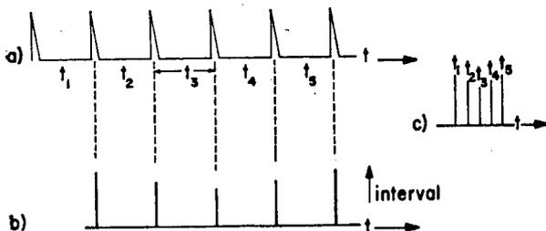
Figure 1—(a) Simulated QRS spike of the EKG. Note difficulty in discerning difference in intervals  $t_1, t_2$ , etc. (b) Interval converted to amplitude. Notice ease in discerning changes. (c) Same as (b) above, except recording speed is reduced for greater readability.
