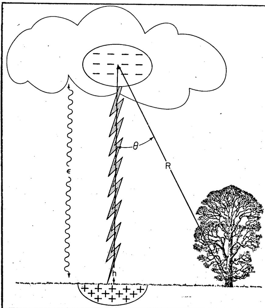
Fig 9. — A diagram showing the electrical situation prior to a lightning stroke. The symbol  $\epsilon$  is the potential difference in the air between the thundercloud and the sky. The + and - symbols indicate the relative charge situation. The symbol  $h$  is the height of the cloud above the ground. The parameter  $R$  is the distance of an object of interest from the stroke and is a function of the angle  $\theta$ .
