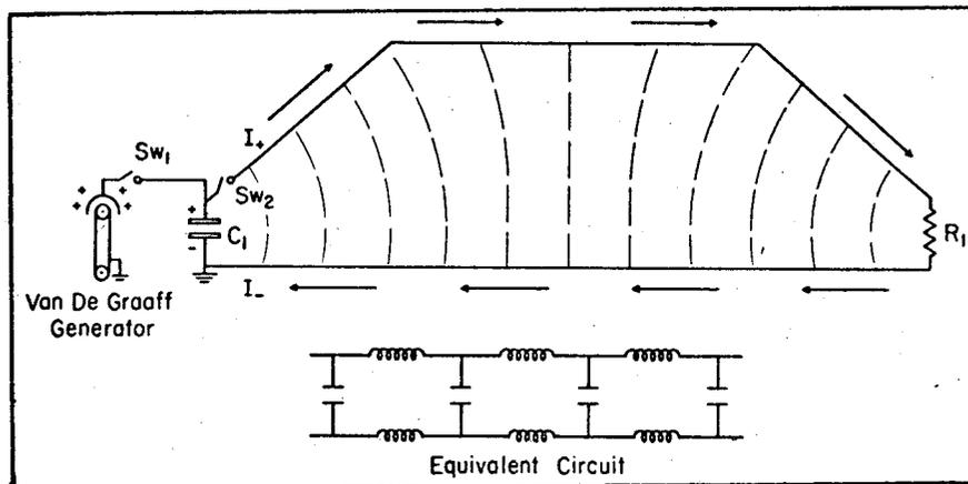
Fig 3. - Circuit diagram and equivalent circuit of a typical EMP generator.
