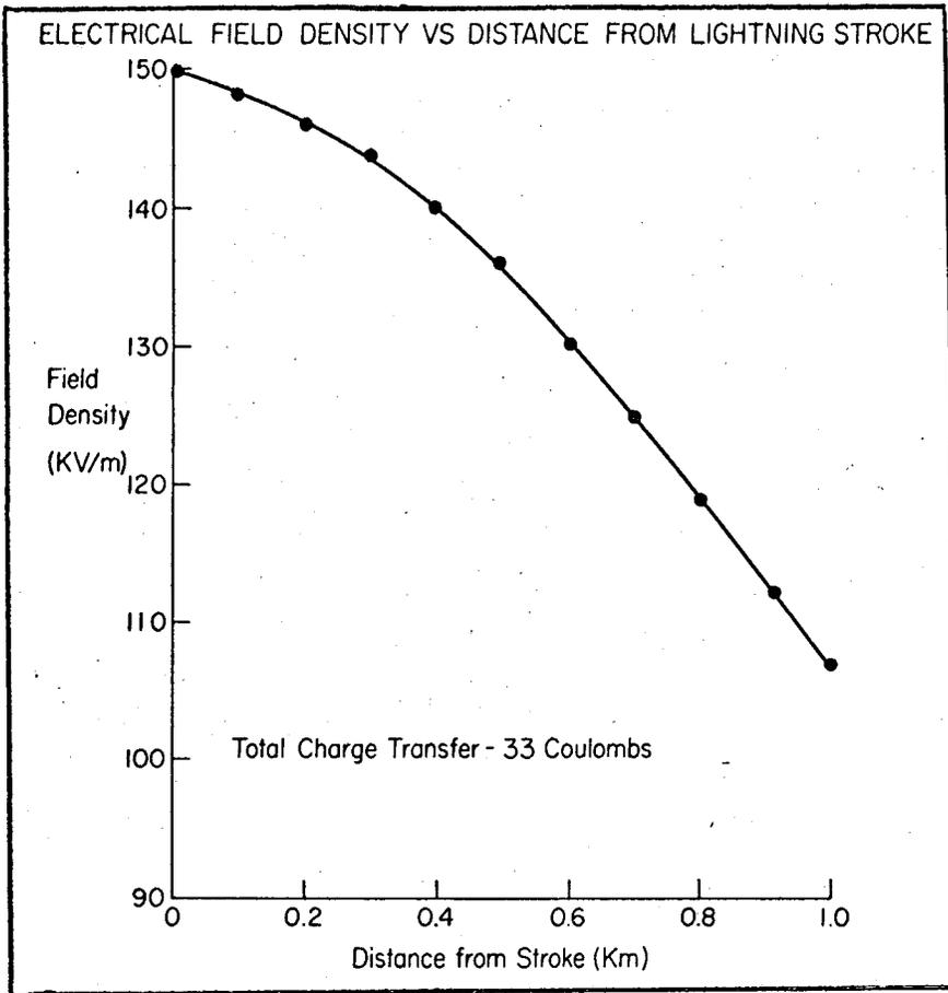
Fig 12. - Electrical field density (E) vs. distance from a typical lightning stroke using data for only the first kilometer.
