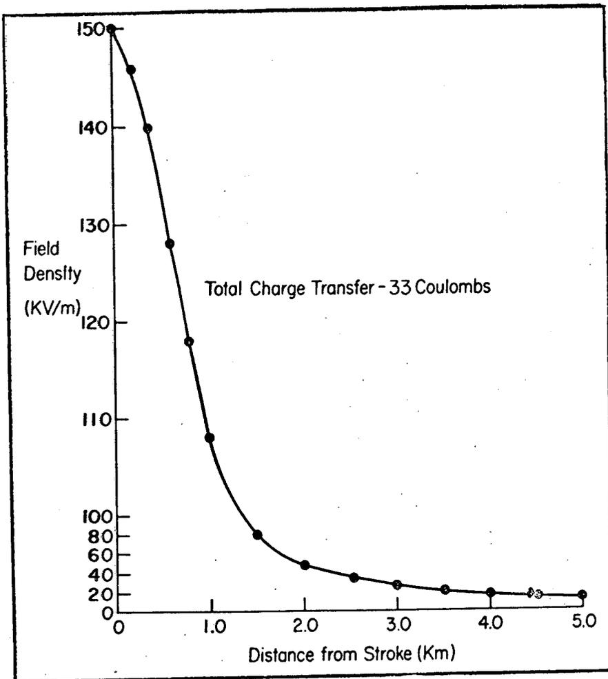
Fig 10. - The equation derived by D. J. Malan to calculate the charge transferral during a lightning stroke. The average stroke transfers 33 coulombs. Using the parameters depicted in Fig 10, the equation can be solved for  $\Delta E$ .
