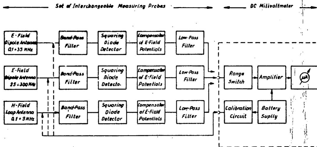
Fig. 3. Block-diagram of a portable instrument for measuring intensities of both electric and magnetic fields.
