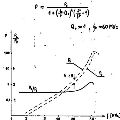
Fig. 1. The absorbed power as a function of frequency for a cylinder simulating a human body when exposed to 1) a distant source and 2) a field in a parallel-plate capacitor.
