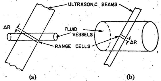
Fig. 2. Fluid flow geometries. (a) Geometry for measuring average flow. (b) Geometry for measuring point velocities.
