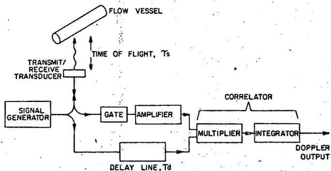
Fig. 1. Correlation system which can model random as well as deterministic Doppler systems.
