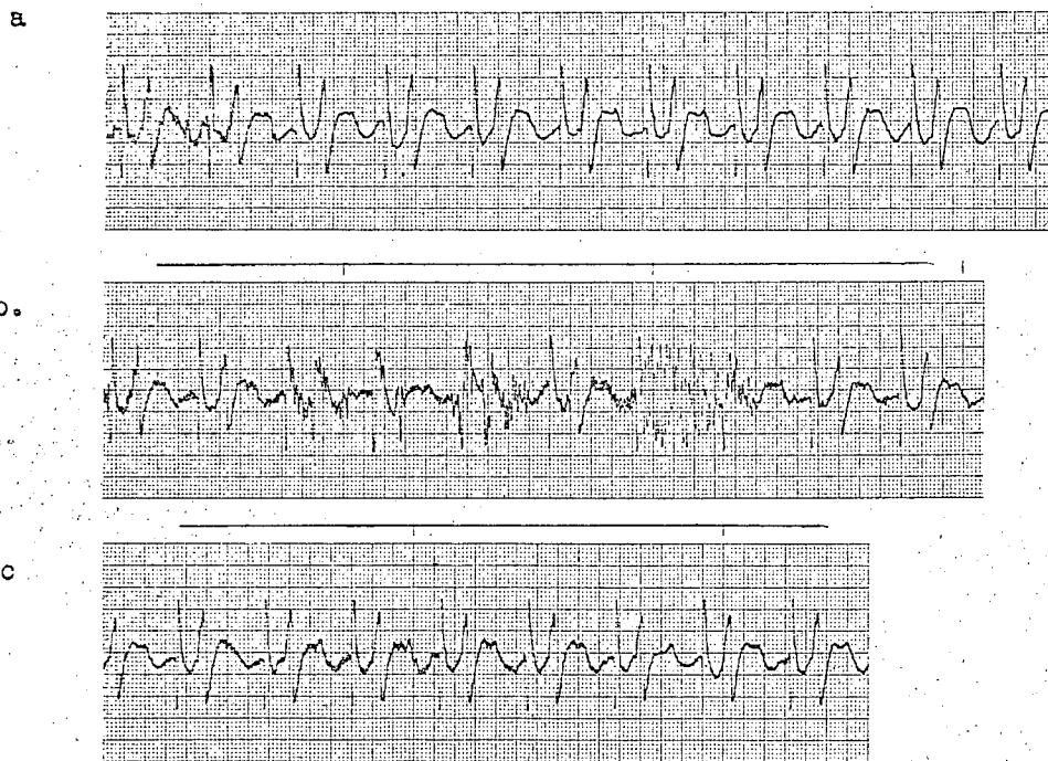
Fig. 10. ECG tracings (Sensitive Ectocor, P-S standby atrial pacing): a. Outside weapons detector. b. In weapons detector—"All Pass"—(No filter). c. In weapons detector—"Filter In." No rate change is noted on clear tracing.
