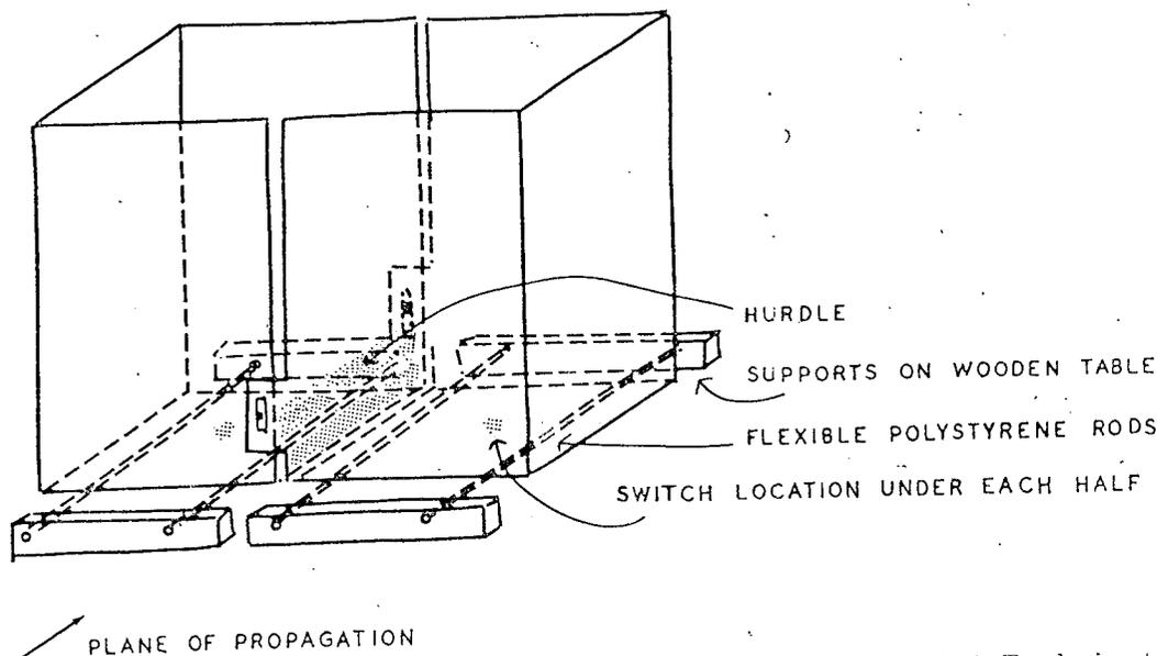
FIGURE 1. Shuttle boxes used in Experiment 1. (Each half was  $22 \times 21 \times 30$  cm. high. Two horizontal polystyrene rods near the top supported a perforated acrylic lid on each half.)
