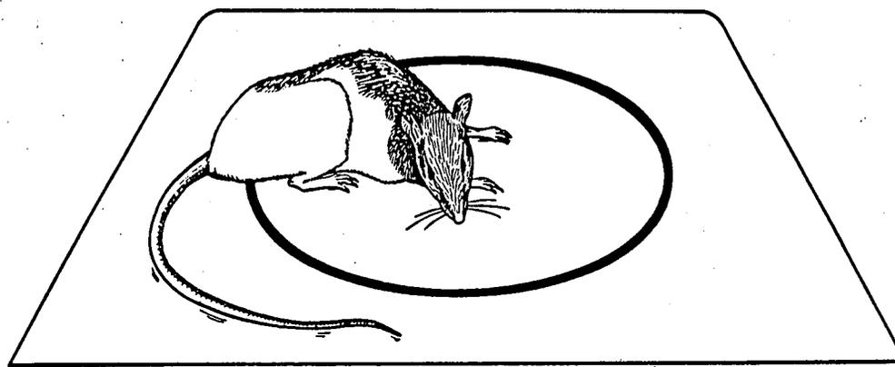
Figure 1. Artist's rendering of a Long-Evans' rat on a false Plexiglas floor that was installed in a 2450-MHz multimode cavity. The circular area described by the black border was centered on the floor and comprised 25 percent of the floor's surface. In the two experiments presented in this paper, entry to the circle by a mouse or rat resulted in cessation of microwave irradiation; exit from the circle, immediate resumption of irradiation.
