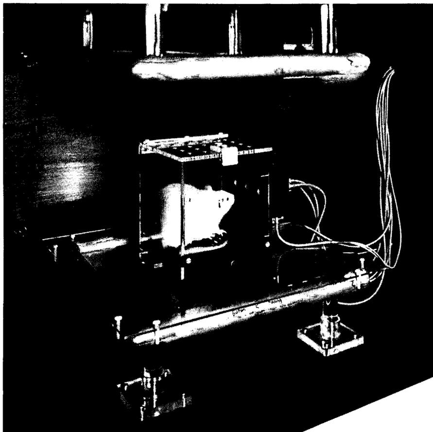
Figure 1. One of the four test chambers that was used in the paradigmatic 60 Hz experiment is illustrated. The fields are established between the aluminum plates positioned on Plexiglas posts above and below the test chamber. Seen above the subject's head are the three lights indicating the positions of each of the three response levers. Extending to the right of the test chamber are the plastic fiber optic guides used for illumination and sensing of presses and the water delivery tube.
