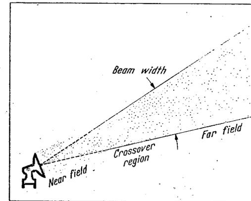
Fig. 1. Radar beam, showing conditions near antenna. "Taken from H. S. OVERMAN"
