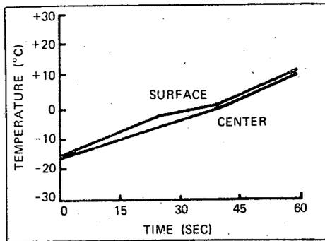
Fig. 4 Temperature of continuously rotated frozen rabbit kidney as a function of time when radiated with 1000 W CW power at 2450 MHz.
