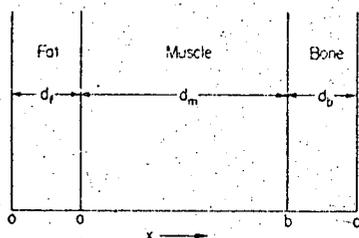
Fig. 1. Analytical model for thermal diffusion.  $H_i(x)$  = thermal source function,  $C_i(x, t)$  = cooling function,  $\rho_i$  = density of the tissue,  $S_i$  = specific heat,  $\kappa_i$  = thermal conductivity,  $k_i$  = diffusion constant ( $i = f, m, b$  for fat, bone, and muscle, respectively).
