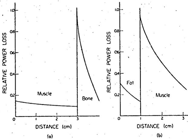
Fig. 2. Relative power loss by (a) ultrasound and (b) microwave. The relative power loss is the power per unit volume converted into heat and normalized to the maximum value.
