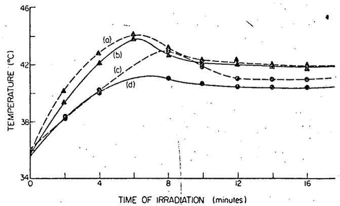
Fig. 7. Temperature rise in human thigh as a function of time (915-MHz microwave radiation). (a) and (c) Experimental results. (b) and (d) Calculated results.
