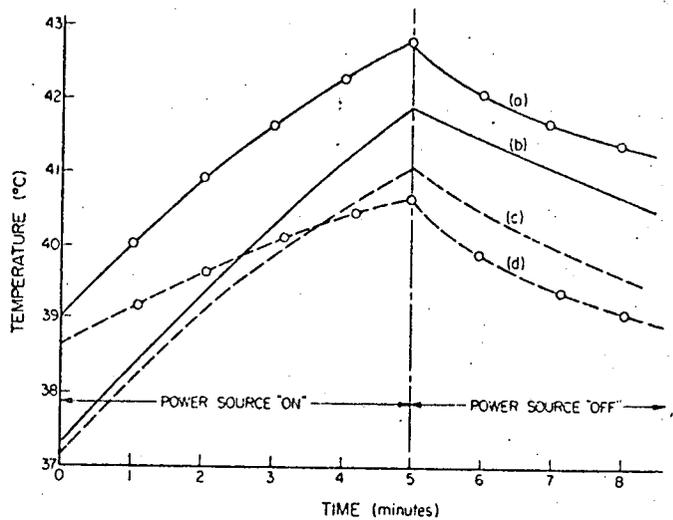
Fig. 6. Calculated and experimental results of the temperature rise as a function of time. The location of the thermocouple is at the bone surface. (a) Experimental temperature without cooling. (b) Calculated temperature without cooling. (c) Experimental temperature with cooling. (d) Calculated temperature with cooling.
