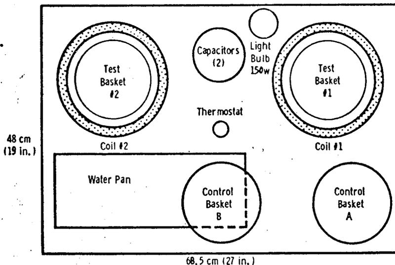
Figure 1.—Incubator diagram for exposing fertilized chicken eggs to 26-kHz, 160-gauss peak to peak a-c field.
