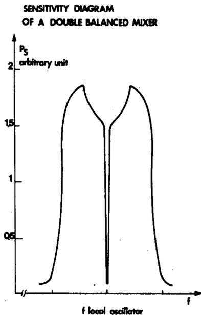
Fig. 4. Typical sensitivity diagram of a double balanced mixer.
