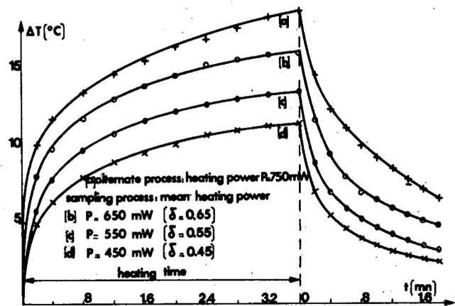
Fig. 5. Temperature variations versus time in minutes for different experimental conditions. (a) Alternating process. (b), (c), (d) Sampling process.
