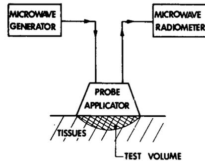
Fig. 1. Block diagram of a microwave heating and radiometry system.
