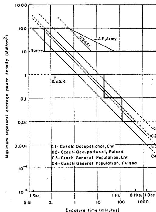
Fig. 1 Maximum Permitted Exposure (Average Power Density) as a Function of Exposure Duration for Several Microwave Radiation Safety Standards on Exposure.
