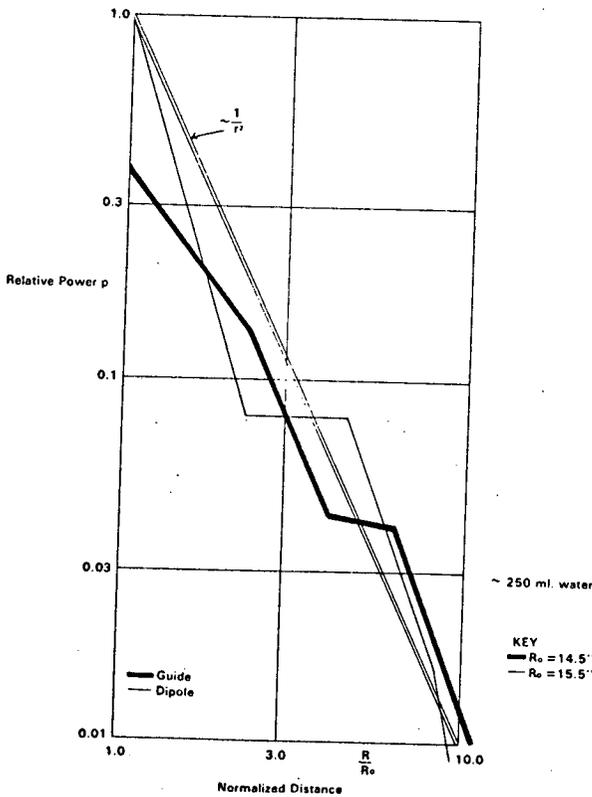
Fig. 3 Relative Level of Microwave Oven Leakage as a Function of Distance from Oven.
