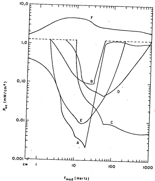
Fig. 5 Critical Power Density Required for Inhibition of Several Models of Demand Pacemakers at 2450 MHz as a Function of Modulation Frequency.
