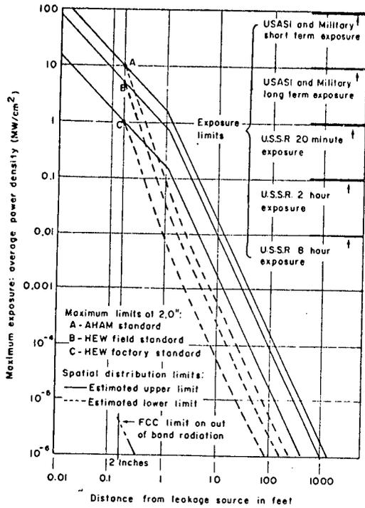
Fig. 2 Estimated Spatial Distributions of Exposure (Average Power Density) Associated with the Principal Microwave Oven Leakage Performance Standards.
