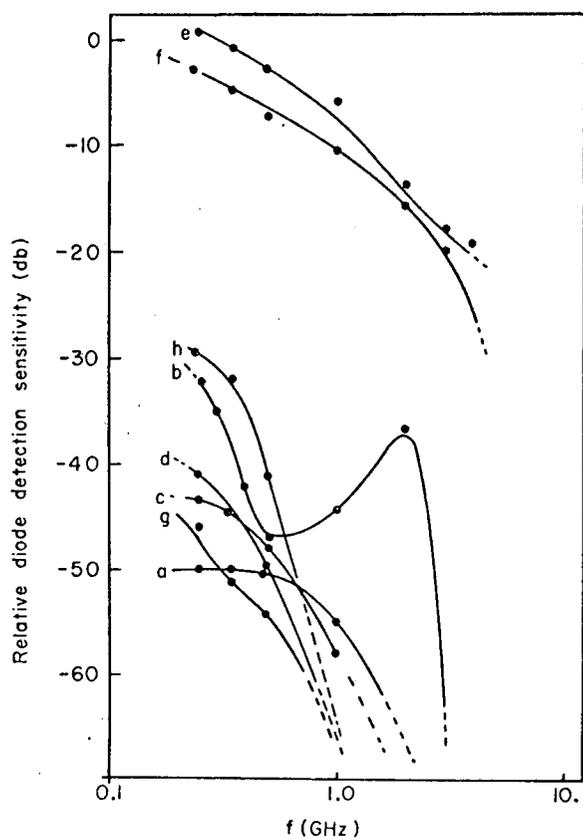
Fig. 6 Relative Diode Detection Sensitivity of Several Semiconductor Components used in Pacemakers, Consumer Products, and Laboratory Instruments as a Function of Frequency: (a) NPD400 diode, (b) IN914 diode, (c) NPD200 diode, (d) 2N4413 transistor, emitter-base, (e) IN295 diode, (f) IN60 diode, (g) 2N3855A transistor, emitter-base, (h) 2N3855A transistor, base-collector.
