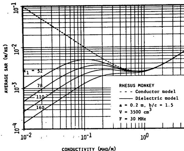
Fig. 3. Averaged specific absorption rate in the ellipsoidal model of a rhesus monkey as a function of the complex dielectric constant at 30 MHz. Incident power density is  $1 \text{ mW/cm}^2$ .
