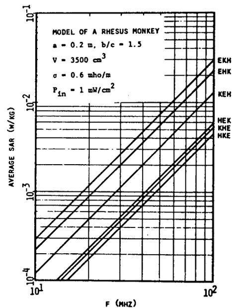
Fig. 6. Averaged specific absorption rate in the ellipsoidal model of a sitting monkey for the six standard polarizations.  $a = 0.2 \text{ m}$ ,  $V = 0.0035 \text{ m}^3$ ,  $b/c = 2$ ,  $\sigma = 0.6 \text{ mho/m}$ ,  $P_{in} = 1 \text{ mW/cm}^2$ .
