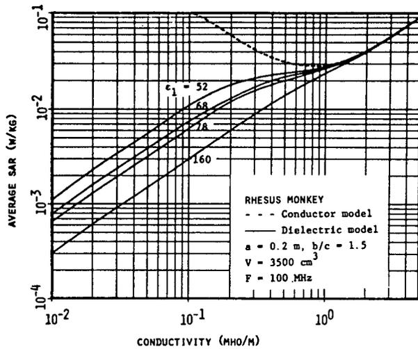
Fig. 4. Averaged specific absorption rate in the ellipsoidal model of a rhesus monkey as a function of the complex dielectric constant at 100 MHz. Incident power density is  $1 \text{ mW/cm}^2$ .
