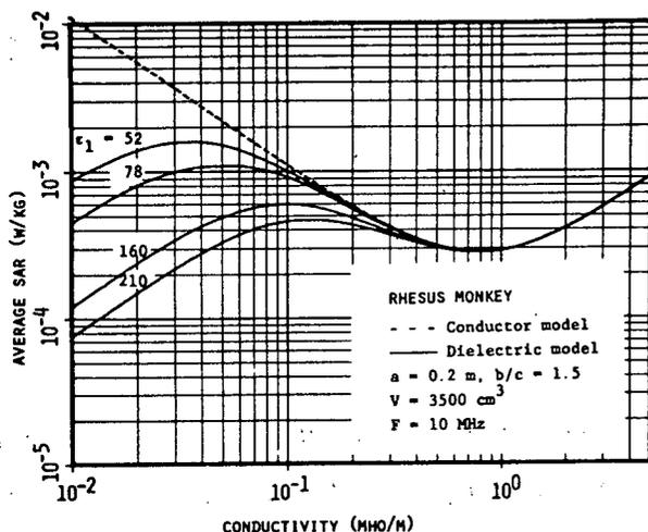
Fig. 2. Averaged specific absorption rate in the ellipsoidal model of a rhesus monkey as a function of the complex dielectric constant at 10 MHz. Incident power density is  $1 \text{ mW/cm}^2$ .
