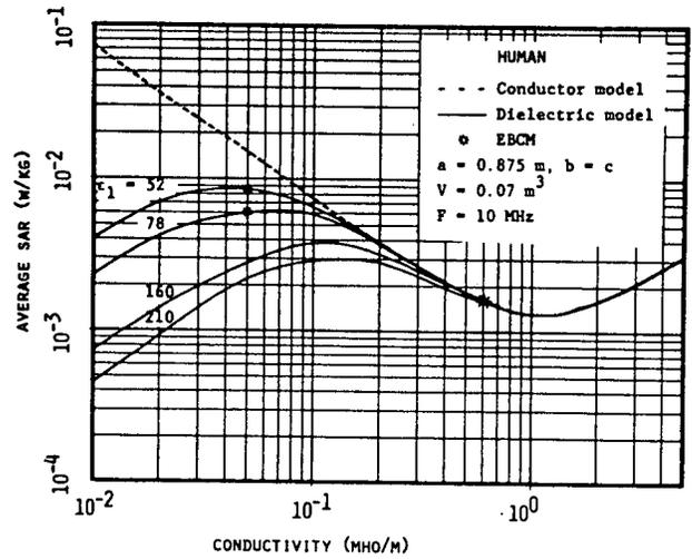
Fig. 5. Averaged specific absorption rate in the prolate spheroidal model of an average man as a function of the complex dielectric constant at 10 MHz. Incident power density is  $1 \text{ mW/cm}^2$ .
