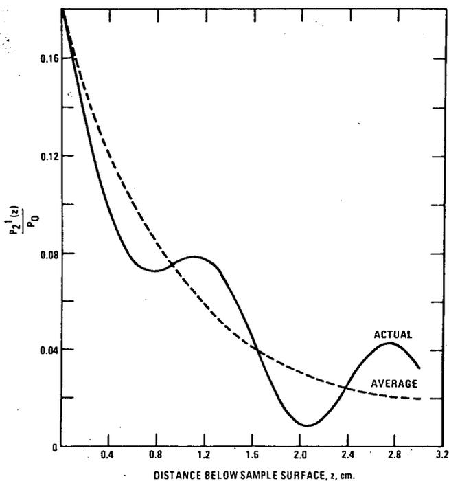
FIG. 4. Normalized power transfer along axis of cell. The ratio of instantaneous power distribution in the sample to incident power is represented as a function of distance below the surface of the sample.
