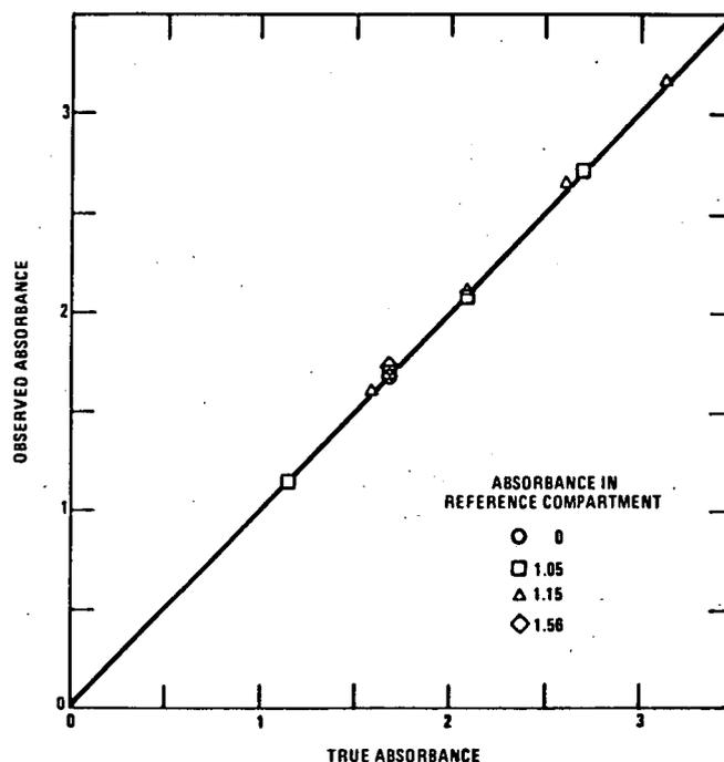
FIG. 5. Stray light measurement. The observed absorbance plotted vs true absorbance shows no negative deviation from Beer's law (line) to  $A=3.1$ .
