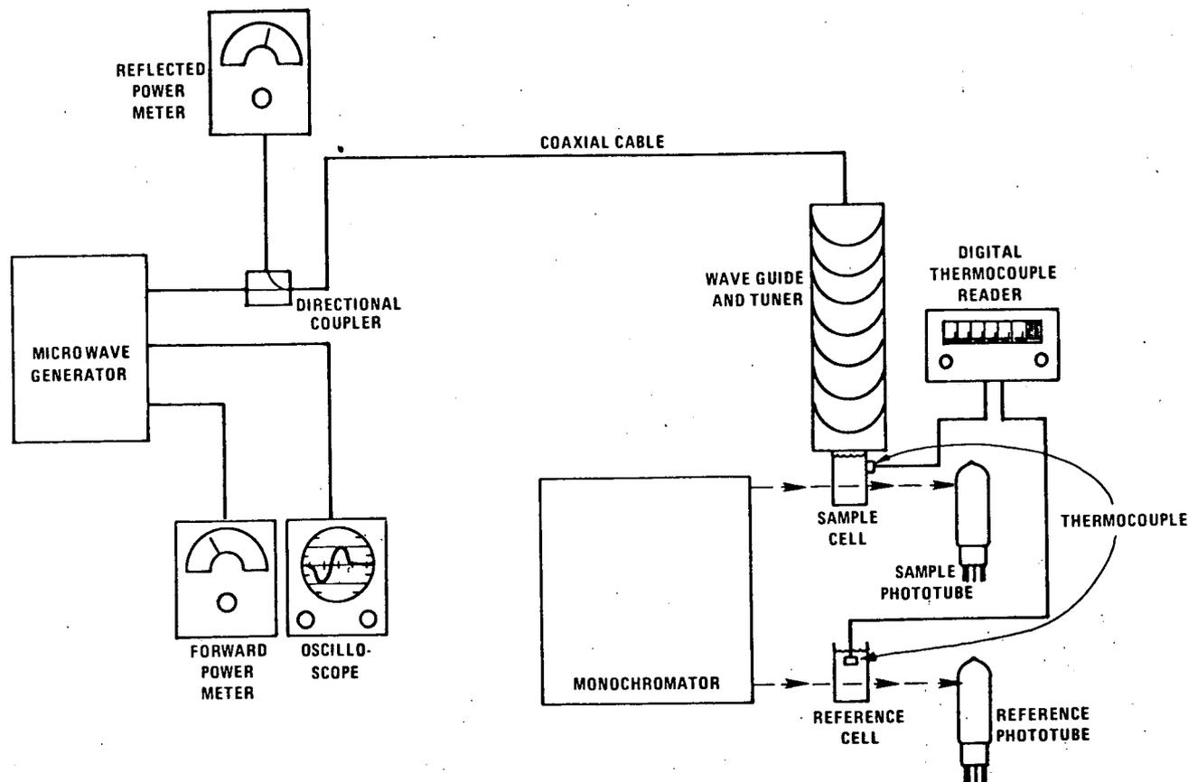
FIG. 1. Schematic of crossed-beam apparatus. The spectrophotometer is represented by a monochromator and phototubes only for simplicity.
