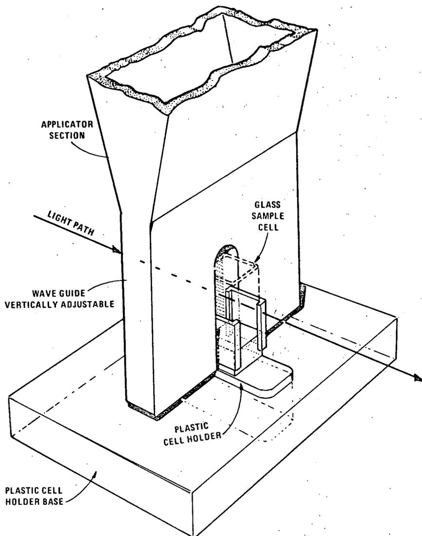
FIG. 2. Applicator and sample cell. The sample cell, held by the plastic cell holder, is illustrated partially inserted under the microwave applicator.
