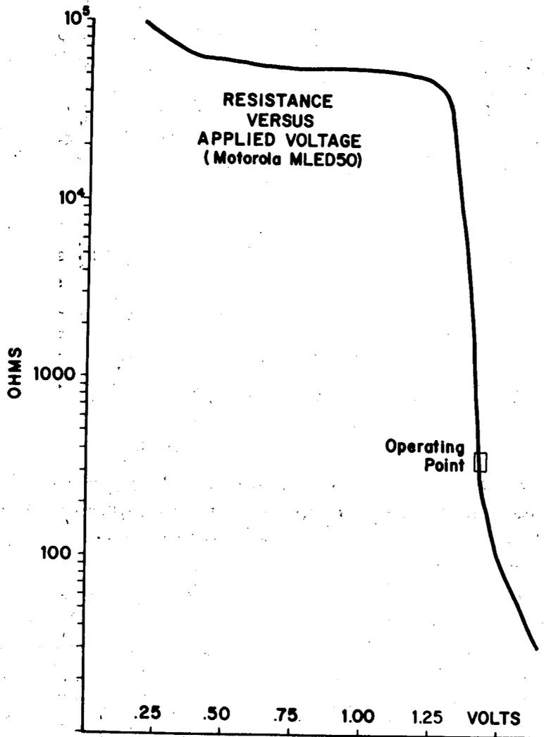
Figure 2. Operating resistance of an LED.
