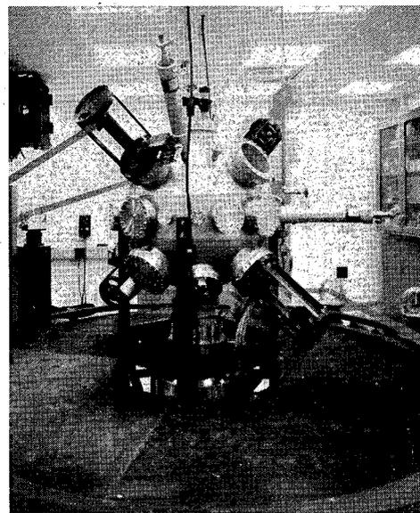
2. The evacuated test chamber shown here houses the target pellet. Cw alignment beams illustrate the paths taken by the four firing pulses.
