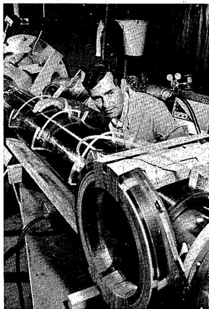
1. This 22-liter HF laser is fired by an electron-beam accelerator visible in the background.
