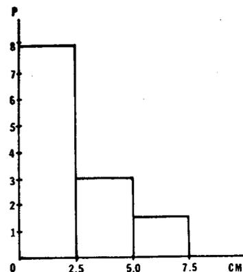
Fig. 4. Power  $P$  in watts, absorbed by physiological saline cylinders of 17.5-cm diameter, 2.5-cm thickness at different distances from the treatment head.
