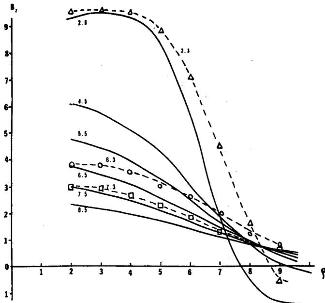
Fig. 1. Spatial variation of the peak axial component  $B_z$  of the magnetic field of a current loop, for  $I = 120$  amperes, peak;  $R = 6.5$  cm;  $\omega = 1.7 \times 10^8$ . The distances in centimeters from the current loop are noted for each curve. The dashed curves are experimentally determined ones.
