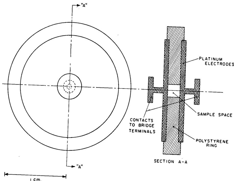
FIG. 2. Cell for dielectric measurement. For description see text.
