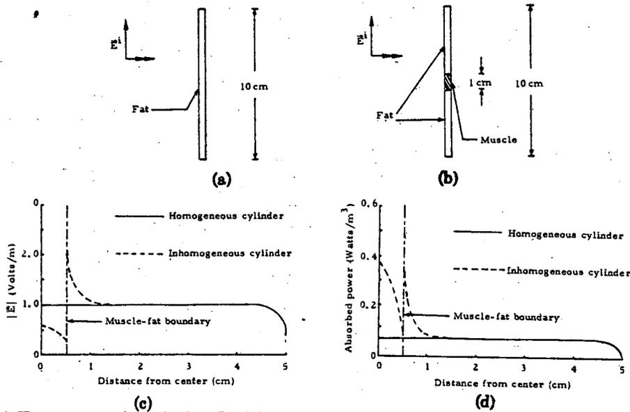
Fig. 9. (a) Homogeneous fat cylinder. (b) Inhomogeneous fat cylinder. (c) Electric field along cylinder axis.  $E^i$  is 1 V/m. (d) Power density ( $1/2\sigma |E|^2$ ) along cylinder axis. Each cylinder was partitioned lengthwise into 100 subvolumes of equal size.
