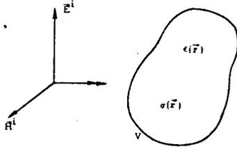
Fig. 1. An arbitrarily shaped biological body illuminated by a plane electromagnetic wave.
