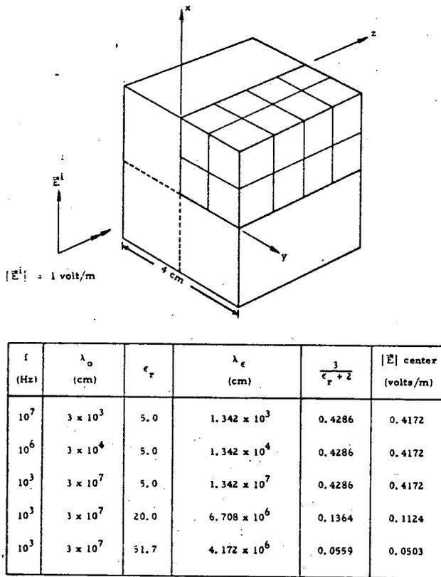
Fig. 3. Electric field at the center of a dielectric cube ( $4 \times 4 \times 4$  cm) induced by plane waves of various frequencies.
