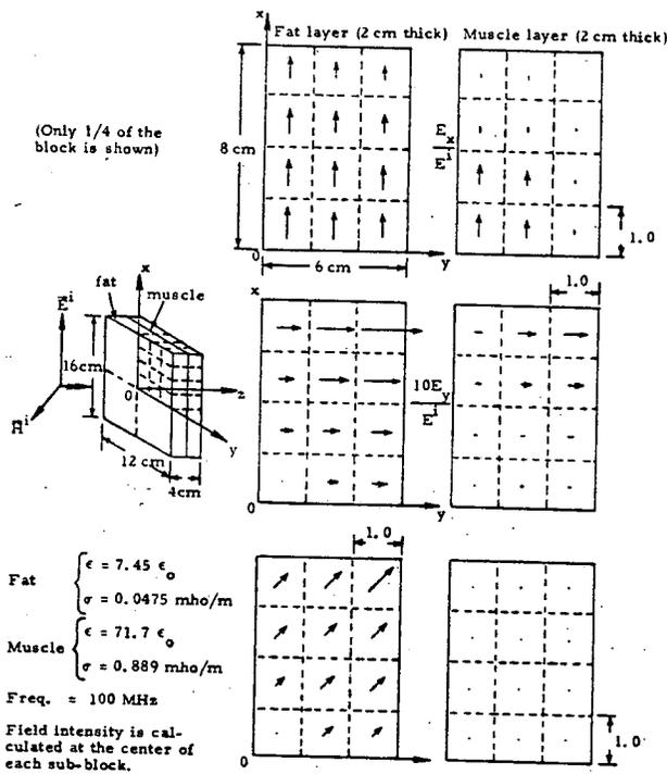
Fig. 6. Distribution of induced electric field inside of a tissue block (16 × 12 × 4 cm) consisting of a fat and a muscle layer. The incident plane wave is  $E = xE^i$  with a frequency of 100 MHz. The field intensity in a corresponding infinite slab model is  $E_z = 0.197E^i$  at the center of the fat layer and  $E_z = 0.210E^i$  at the center of the muscle layer.
