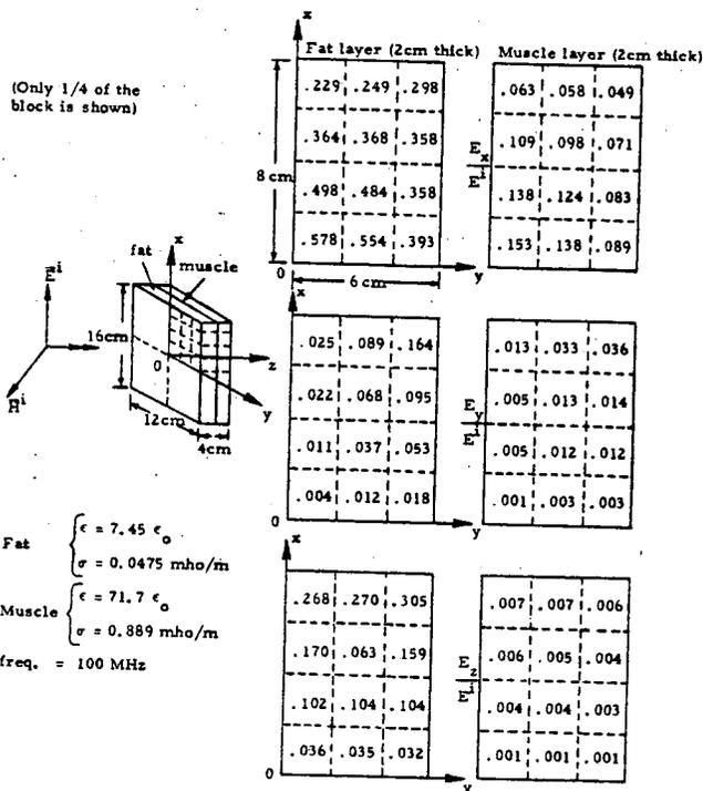
Fig. 7. Distribution of induced electric field inside of a tissue block (16 × 12 × 4 cm) consisting of a fat and a muscle layer. The field intensity is calculated at the center of each subblock. For a corresponding infinite slab model  $E_z = 0.197E^i$  at the center of the fat layer and  $E_z = 0.210E^i$  at the center of the muscle layer.
