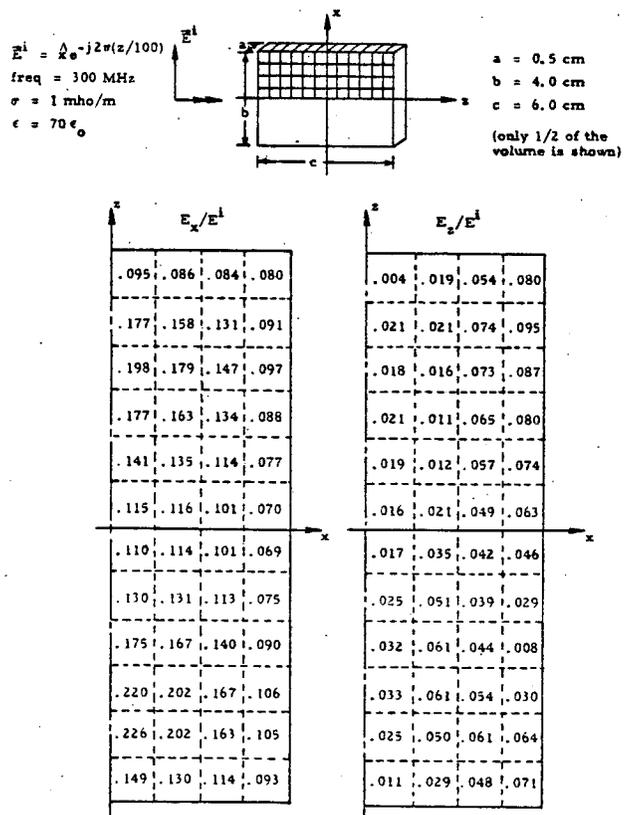
Fig. 5. Electric field inside of a layer of conducting medium with  $\epsilon = 70\epsilon_0$ ,  $\sigma = 1$  mho/m induced by a plane wave of 300 MHz with the incident electric field parallel to the flat surfaces of the layer.
