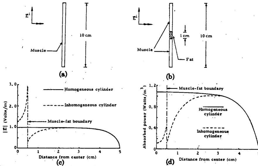
Fig. 8. (a) Homogeneous muscle cylinder. (b) Inhomogeneous muscle cylinder. (c) Electric field along cylinder axis.  $E^i$  is 1 V/m. (d) Power density ( $1/2\sigma |E|^2$ ) along cylinder axis. Each cylinder was partitioned lengthwise into 100 subvolumes of equal size.
