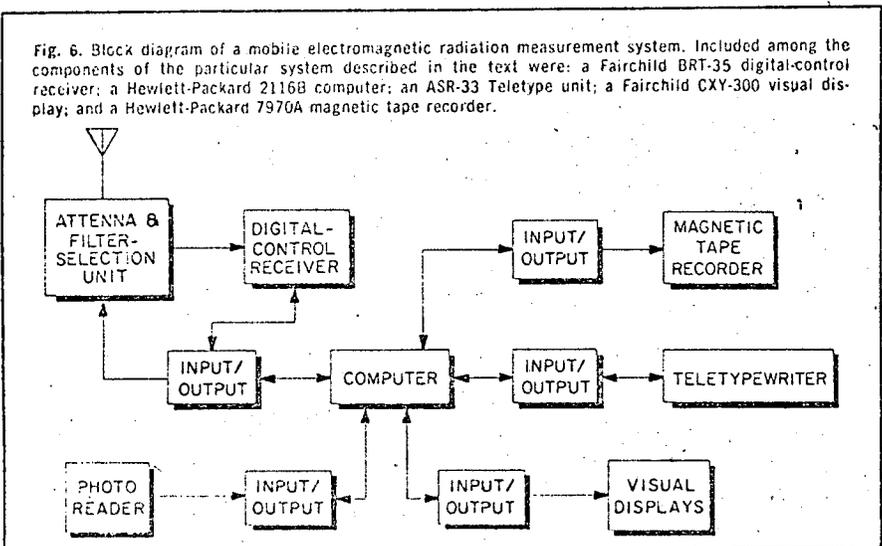
a broad-range, variable-bandwidth receiver (shown in Fig. 5), an on-board computer, a magnetic tape unit, and video display systems.
