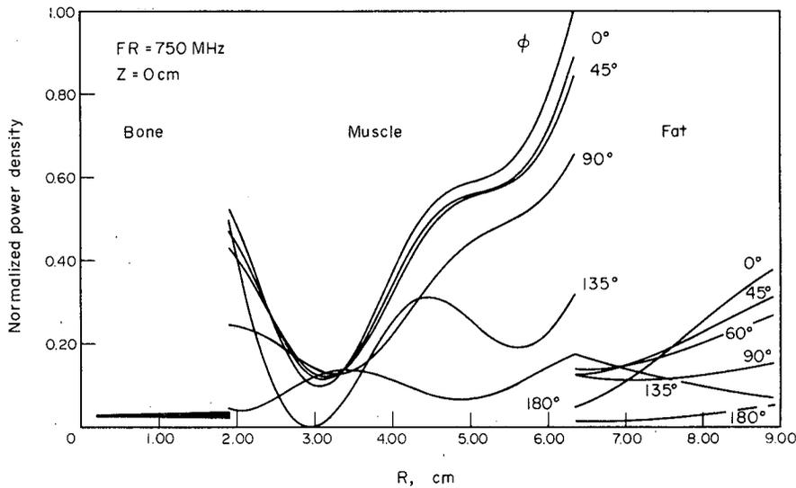
FIG. 8. Absorption patterns of thigh size model with plane wave source  $H_z$  polarization, freq. = 750 MHz.
