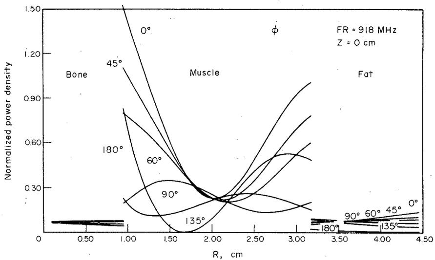
FIG. 15. Absorption patterns of arm size model with plane wave source  $H_z$  polarization, freq. = 918 MHz.
