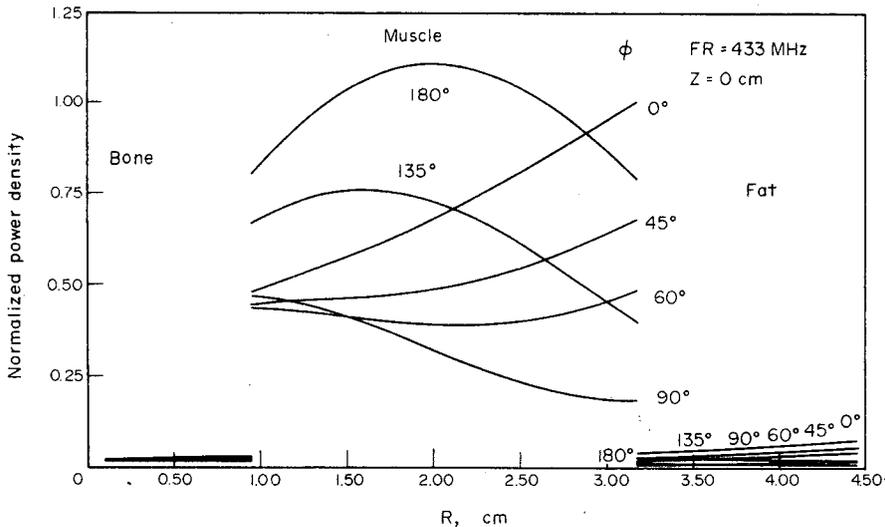
FIG. 13. Absorption patterns of arm size model with plane wave source  $E_z$  polarization, freq. = 433 MHz.
