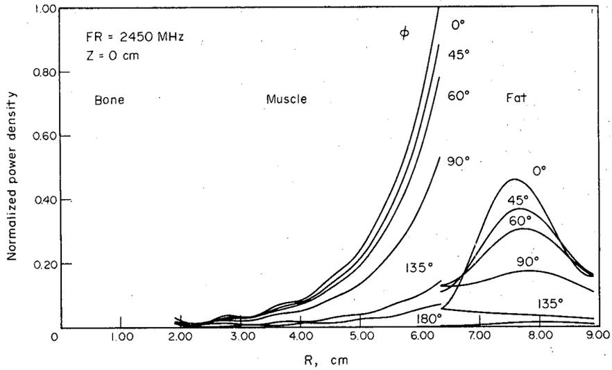
FIG. 6. Absorption patterns of thigh size model with plane wave source  $H_z$  polarization, freq. = 2450 MHz.
