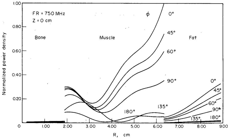
FIG. 4. Absorption patterns of thigh size model with plane wave source  $E_z$  polarization, freq. = 750 MHz.
