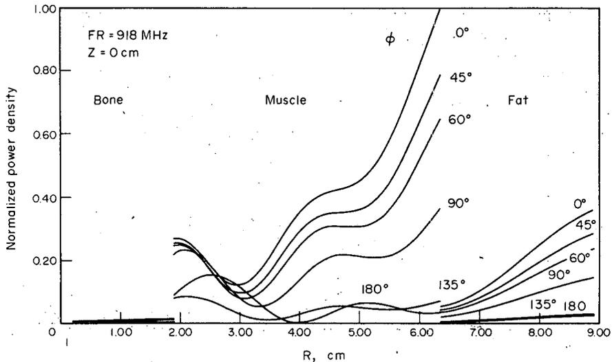
FIG. 3. Absorption patterns of thigh size model with plane wave source  $E_z$  polarization, freq. = 918 MHz.
