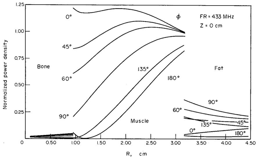
FIG. 17. Absorption patterns of arm size model with plane wave source  $H_z$  polarization, freq. = 433 MHz.
