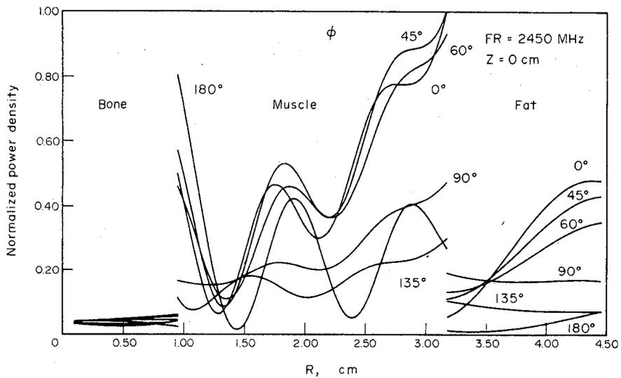
FIG. 14. Absorption patterns of arm size model with plane wave source  $H_z$  polarization, freq. = 2450 MHz.
