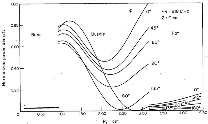
FIG. 11. Absorption patterns of arm size model with plane wave source  $E_z$  polarization, freq. = 918 MHz.
