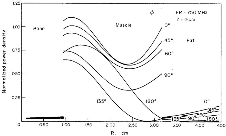
FIG. 12. Absorption patterns of arm size model with plane wave source  $E_z$  polarization, freq. = 750 MHz.
