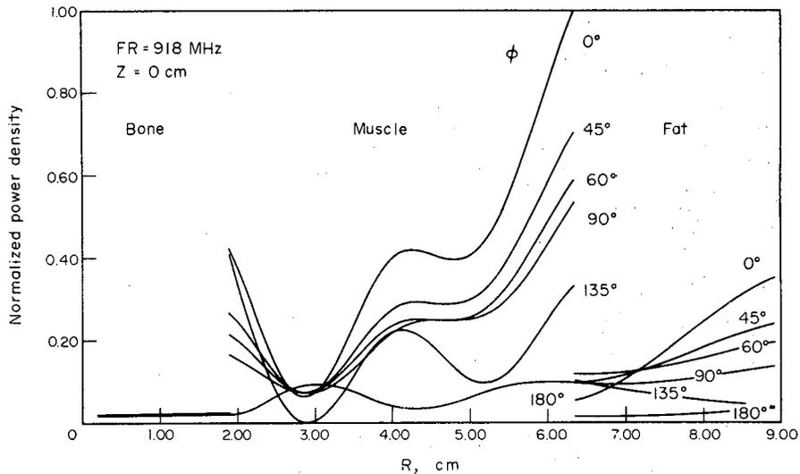
FIG. 7. Absorption patterns of thigh size model with plane wave source  $H_z$  polarization, freq. = 918 MHz.
