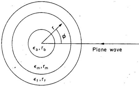
FIG. 1. Plane wave incident on triple-layered dielectric cylinder  $r_b$ ,  $r_m$ ,  $r_f$  and  $\epsilon_b$ ,  $\epsilon_m$ ,  $\epsilon_f$  are respectively the radii and complex dielectric constants of bone, muscle and fat tissue layers.
