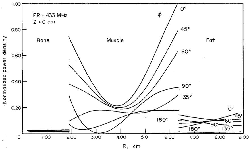
FIG. 9. Absorption patterns of thigh size model with plane wave source  $H_z$  polarization, freq. = 433 MHz.
