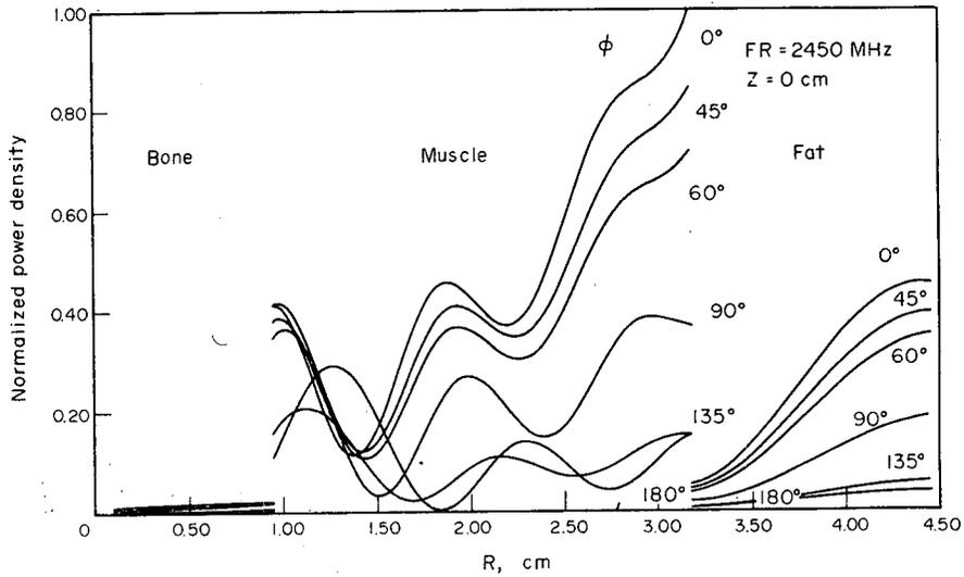
FIG. 10. Absorption patterns of arm size model with plane wave source  $E_z$  polarization, freq. = 2450 MHz.
