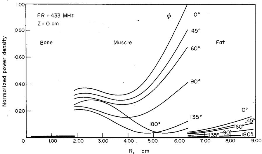
FIG. 5. Absorption patterns of thigh size model with plane wave source  $E_z$  polarization, freq. = 433 MHz.
