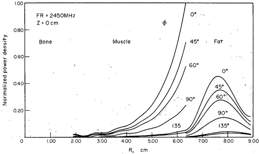
FIG. 2. Absorption patterns of thigh size model with plane wave source  $E_z$  polarization, freq. = 2450 MHz.
