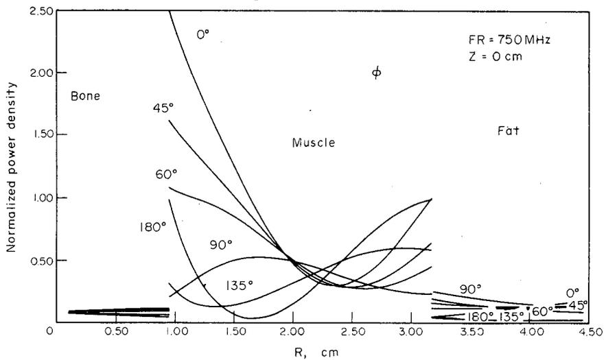
FIG. 16. Absorption patterns of arm size model with plane wave source  $H_z$  polarization, freq. = 750 MHz.
