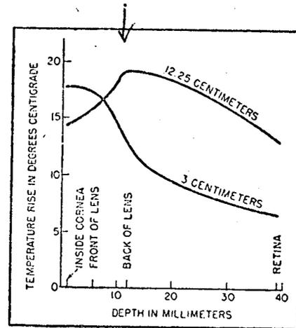
FIG. 1—Experimentally-determined variation of temperature in an excised beef eye exposed to microwave radiation
