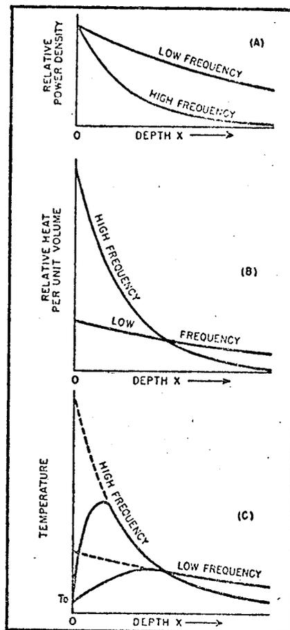
FIG. 2.—Variations with depth in an idealized animal. Curves of (C) are calculated, assuming no cooling due to circulation of blood
