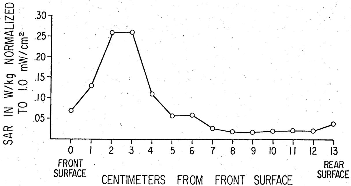
Figure 2. Measured SAR in primate phantom model at 1.29 GHz. All points were located in the sagittal plane on a horizontal line at eye level.
