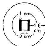
FIG. 3. Schematic of Kerr cell. Cylinder made of high quality Lucite with stainless-steel electrodes.
