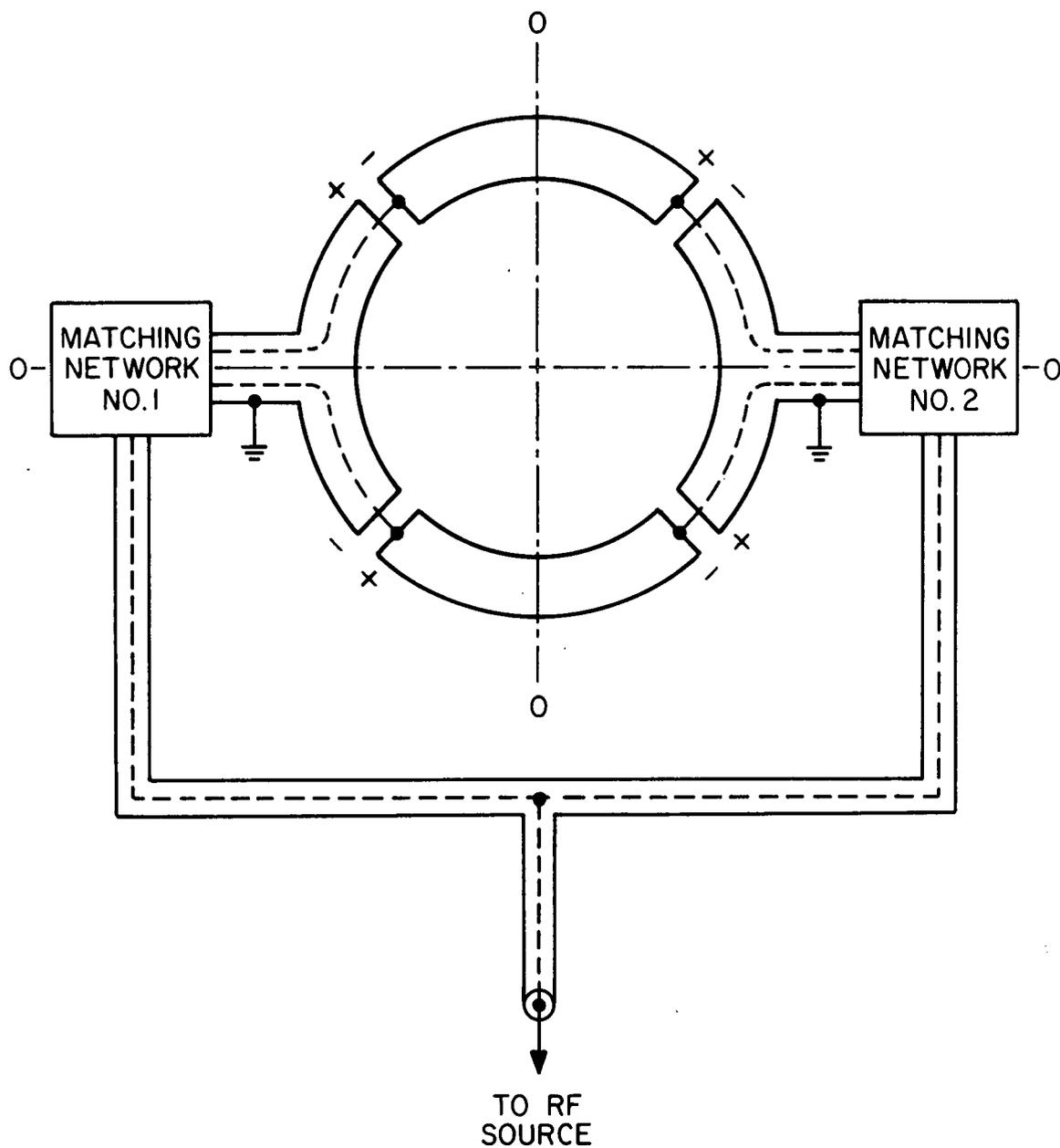
Figure 1. A Block Diagram of the RF Magnetic-Field Generator Showing the Four-Gap Shielded-Loop Inductor and the Associated Tunable Matching Networks for Use from 10 to 40 MHz. The Two Orthogonal Image Planes are Shown Intersecting at the Center of the Loop.
