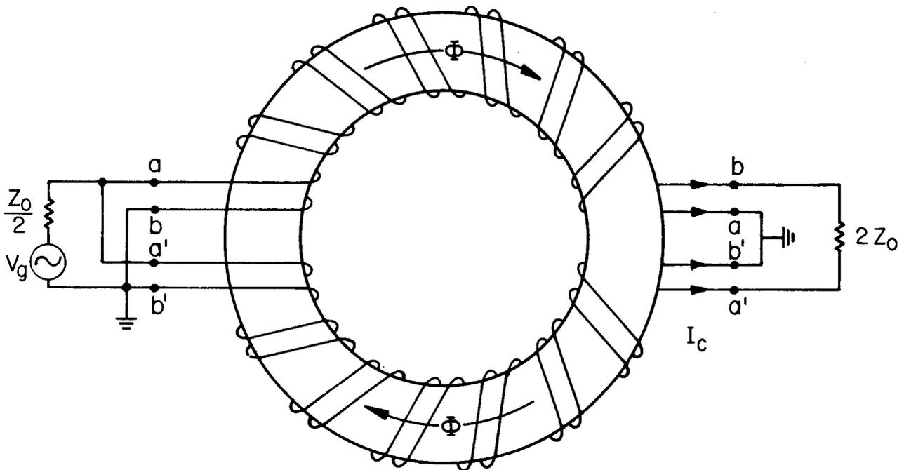
Figure 8. The General Method of Winding Used in the Toroidal Balun Transformer. The Basic Arrangement is the Same as that of Figure 7, Except that the Transmission Lines Have Been Wound on a Toroidal Core to Increase the Common-Mode Rejection at the Lower Frequencies.
