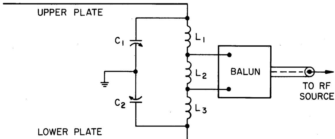
Figure 11. The Circuit Diagram of the Parallel-Plate Matching Network.
