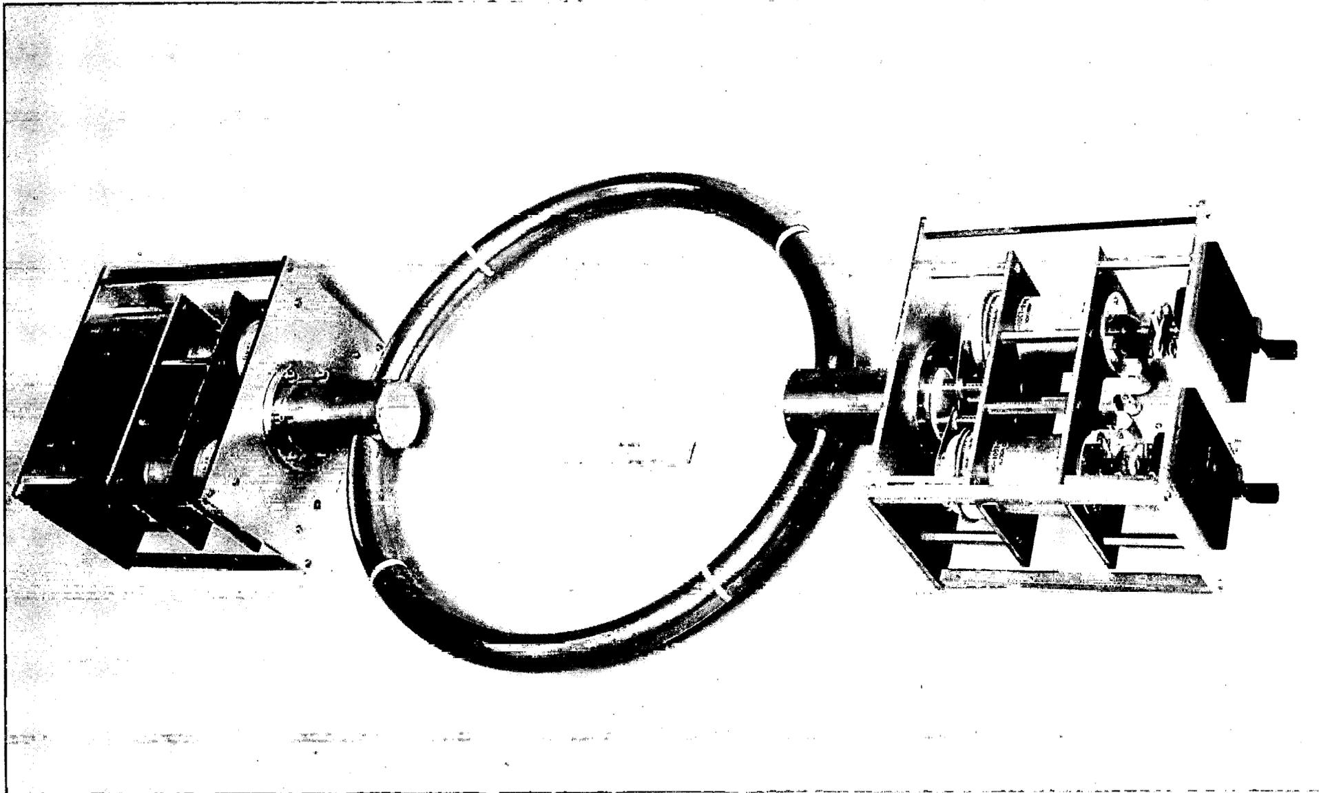
Figure 3. An Assembled View of the RF Magnetic-Field Generator Showing the Shielded-Loop Inductor and the Two Integral Matching Networks with Covers Removed.
