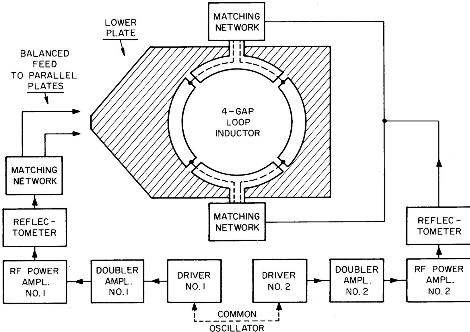
Figure 12. A Block Diagram of the Complete RF Near-Field Synthesizer Showing All of the Principal Components Including the RF Power Sources.
