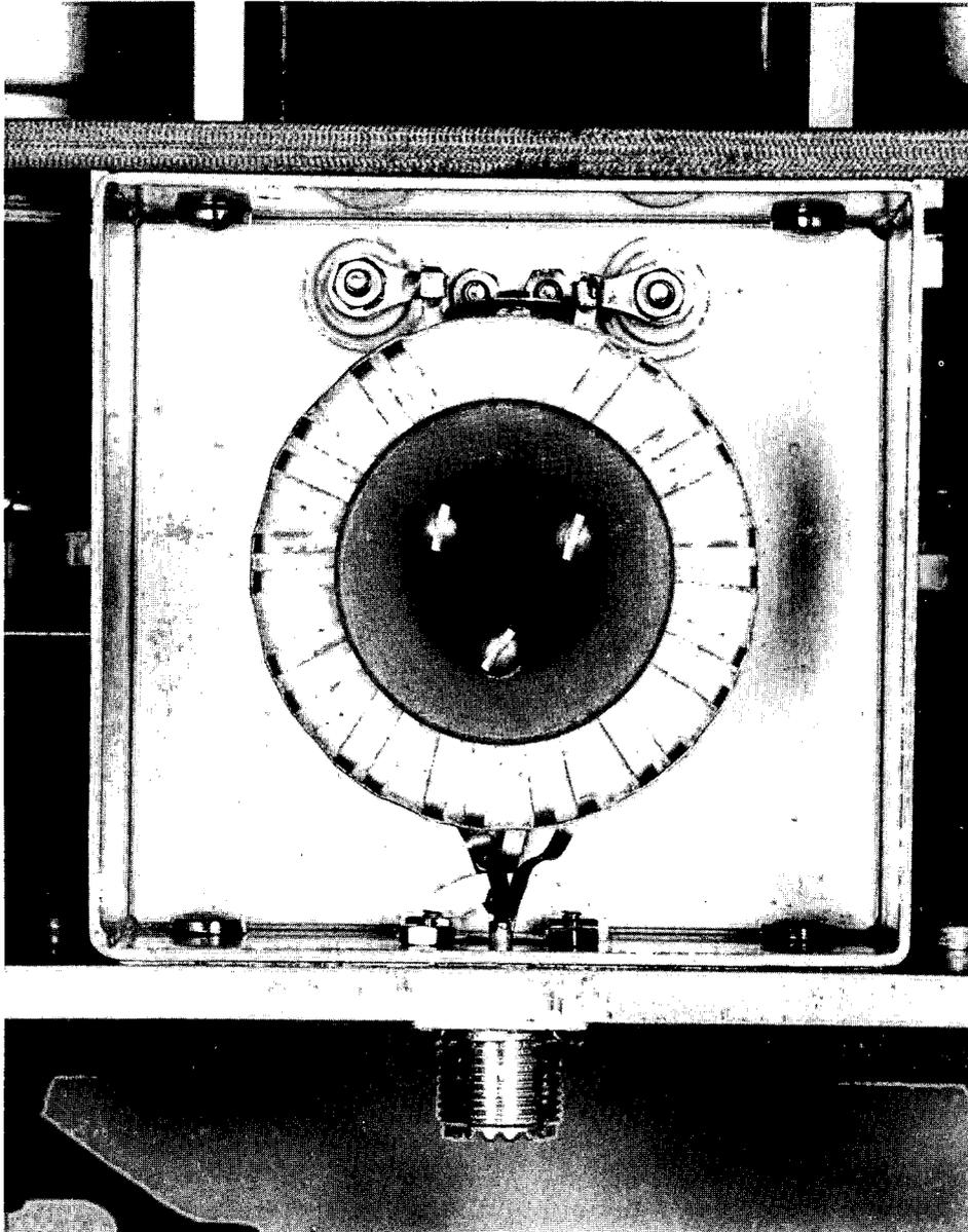
Figure 6. A Bottom View of One of the 75 to 300 Ohm Toroidal Balun Transformers Used in the Loop-Inductor Matching Networks.
