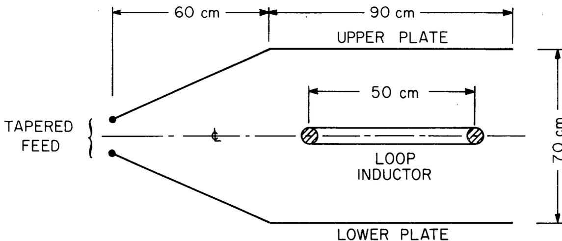
Figure 9. The General Arrangement of the RF Near-Field Synthesizer. The Loop Inductor is Located Midway between the Balanced Parallel Plates Normally in the Neutral Plane, but can be Tilted at Any Angle up to 60 Degrees.
