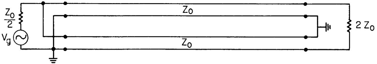
Figure 7. A Basic Balun Circuit Comprising Two Balanced Transmission Lines of Characteristic Impedance,  $Z_0$ . The Lines are Connected in Parallel at One End and in Series at the Other, Giving an Impedance Transformation Ratio of 4:1.
